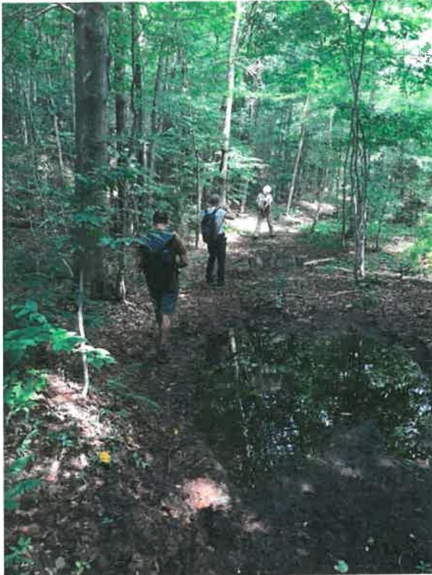
**Photo 13: Large puddle of standing water along a snowmobile trail, indicated the trail route passing through a low-lying wet area with poor drainage.**
